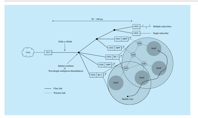
Fig. 1. FiWi enhanced LTE-A HetNet architecture for WiFi offloading.
