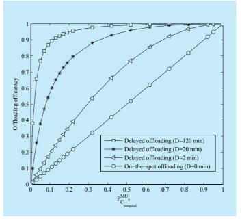
**Fig.2.** Offloading efficiency vs. temporal FiWi connectivity probability of mobile users for on-the-spot and delayed offloading.
