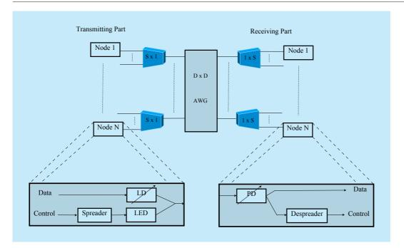
**Fig. 5** Scalable switchless single-hop WDM network using multiple FSRs of a wavelength-routing AWG for east-west flows in data centers.
