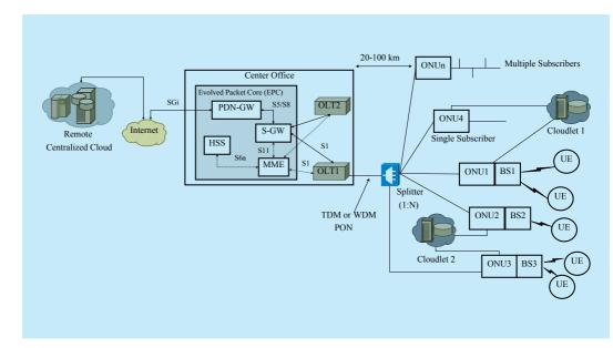
Fig. 4 Cloud and cloudlet empowered FiWi-HetNet architecture.
