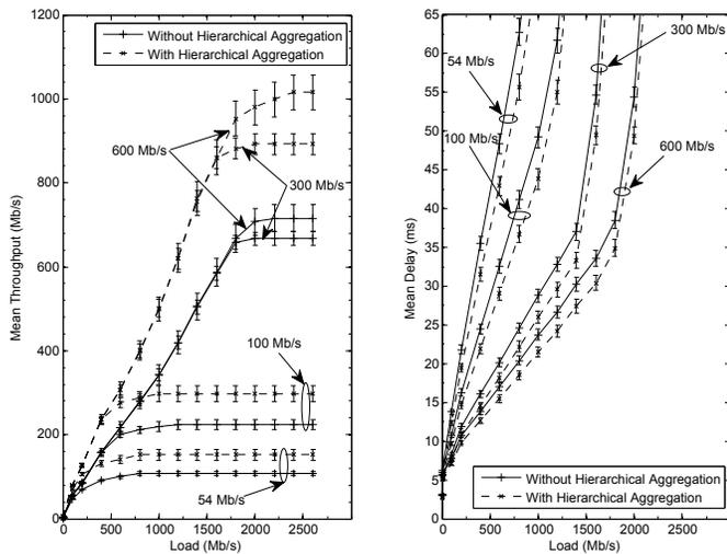
Fig. 5. Impact of hierarchical frame aggregation on integrated EPON-WLAN network performance for various WMN data rates under triple-play traffic.
