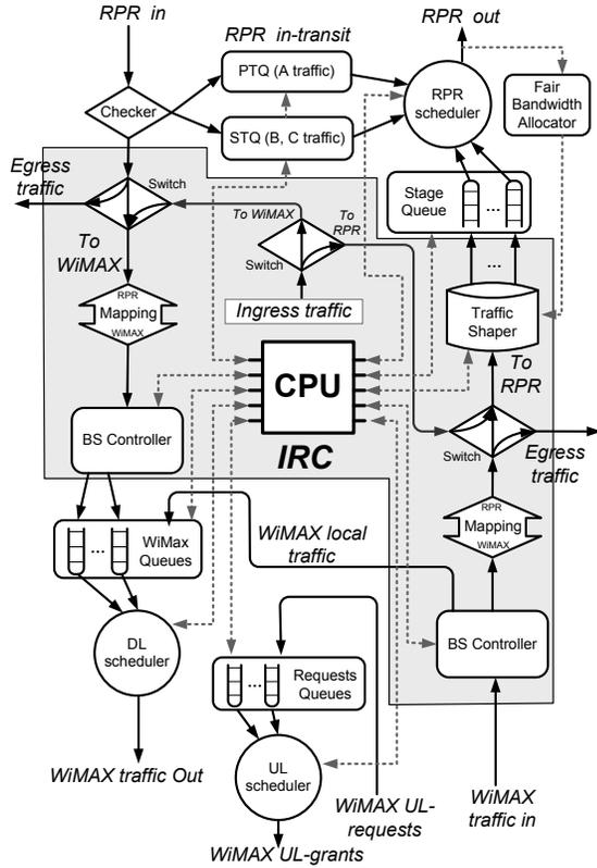
Fig. 1. Optical-wireless interface between RPR and WiMAX networks.
