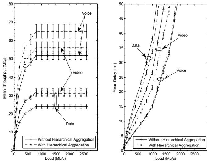
Fig. 4. Impact of hierarchical frame aggregation on integrated EPON-WLAN network performance for a 54 Mb/s WMN under triple-play (voice, video, and data) traffic.
