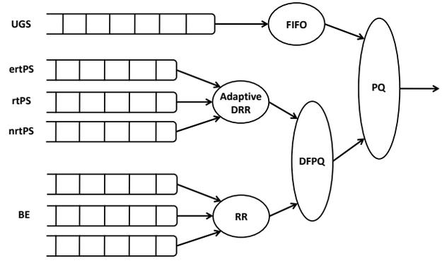
Fig. 2. Hierarchical scheduling algorithm for WiMAX/RPR interface.
